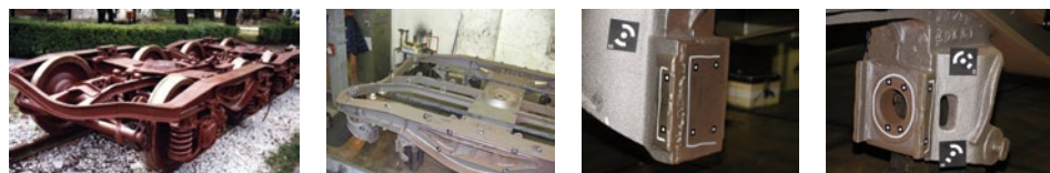
Fig. 4: You can see the finished swivel-truck on the left, the frame with reference points in the middle and two details with marked features on the right.
