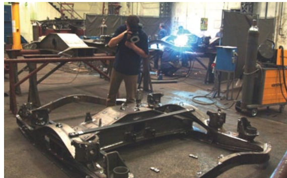
Fig. 5: Taking photos to measure the connection areas and important dimensions of the swivel-truck.
